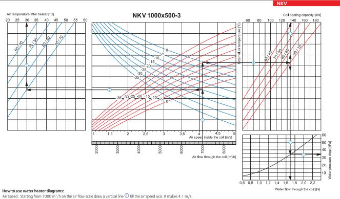
Supply air temperature. Prolong the line 🛈 up to the point where it crosses the outside air temperature (blue curve), e.g. -20 °C; then draw a horizontal line 🖉 from this point to the left till crossing water
