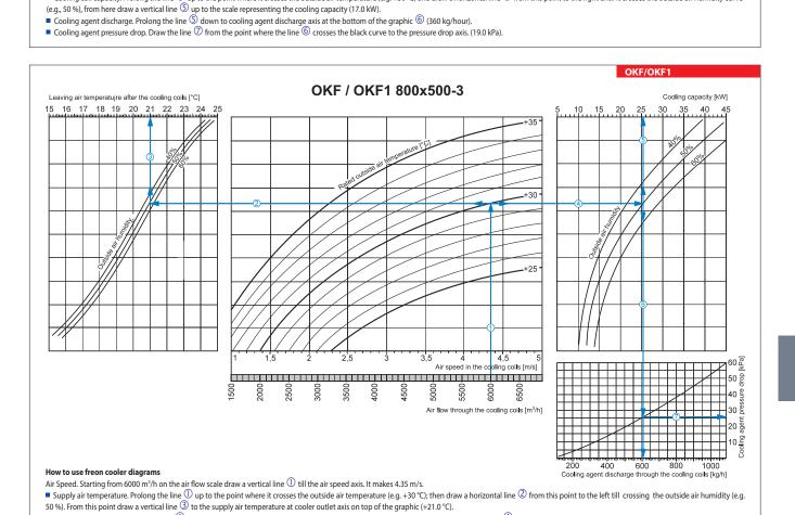
Cooling coil capacity. Prolong the line ① up to the point where it crosses the outside air temperature (e.g. +30 °C) and draw a horizontal line ④ from this point to the right until it crosses the outside air humidity curve
