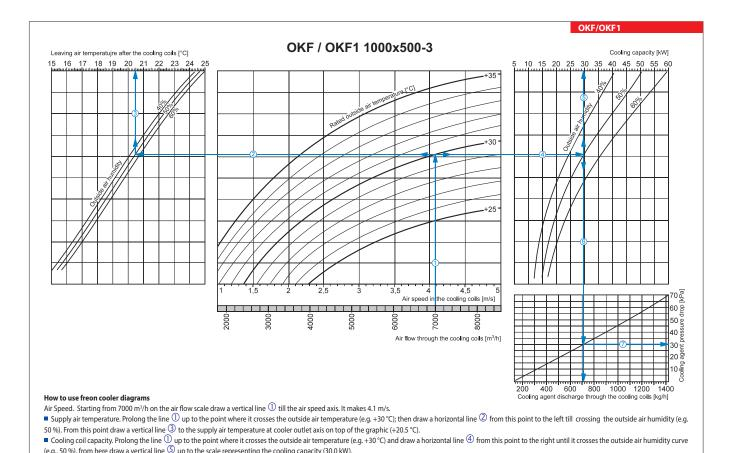
(e.g., 50 %), from here draw a vertical line (5) up to the scale representing the cooling capacity (30.0 kW).
