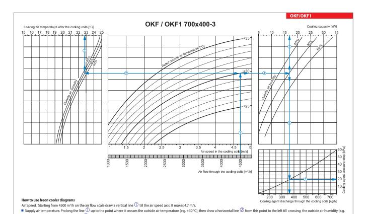
Cooling coil capacity. Prolong the line 🗓 up to the point where it crosses the outside air temperature (e.g. +30 °C) and draw a horizontal line 🕙 from this point to the right until it crosses the outside air humidity curve
