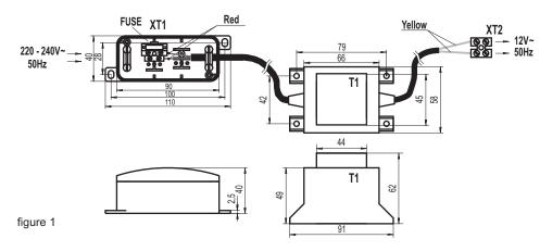
For protection against overloads, the transformer has replaceable fuse FUSE integrated in the input terminal block XT1. For the safety grounds, the terminal block XT1 is mounted in the protective terminal box. The output terminal block XT2 serves for connection of the fan with safe supply voltage of 12 V.
