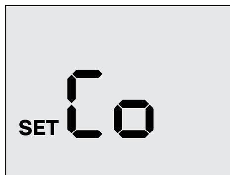
Use the **M** and **↻** buttons to select the parameter code for editing and set the desired value by means of the **▲** and **▼** buttons.
