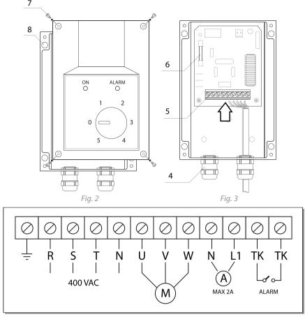
Fig. 4. Connection Diagram
