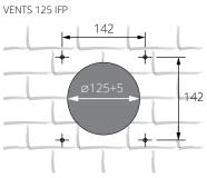
4. Bore dowel holes. Then install the fan using the screws and install the front panel.
