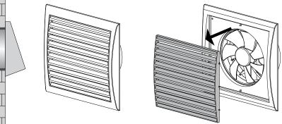
3. Attach the fan to the wall or use the drawings below to mark the holes for dowels. While preparing the holes it's recommended to provide the fan connection and the network cable routing methods.
