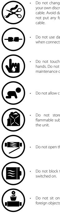
Do not change the power cable length at your own discretion. Do not bend the power cable. Avoid damaging the power cable. Do not put any foreign objects on the power cable.
