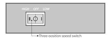
The fan with AC motor is controlled by a three-position switch. The switch has three positions:
