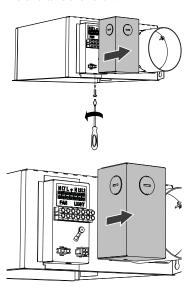
Remove the protective cap and install the cable gland.
