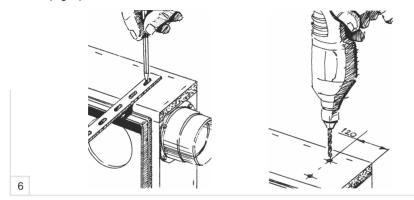
3. Fasten the mounting holders to the casing using universal screws 3.5x16 (Fig. 7).
