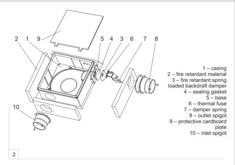
Save the protective cardboard plate 9 (Fig. 2) removed from the KP 80 casing before mounting for reinstallation into the casing after mounting.
