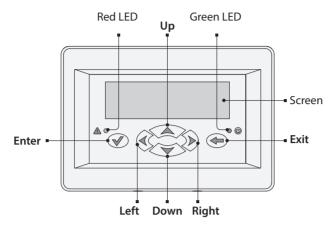
Fig. 2 Control panel button functions
