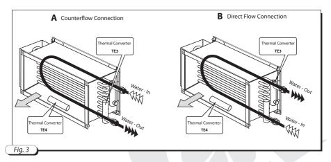
Heat transfer medium connection to the hydronic water coil heater is shown on Fig. 4.
