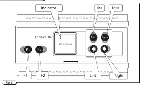
The digital controller is the principal control unit component (Fig. 8).
