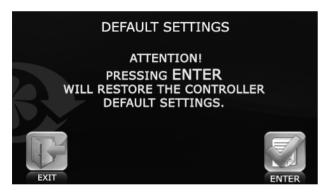
■ To reset the controller settings to the factory defaults select **DEFAULT SETTINGS** submenu from the Engineering menu and press
