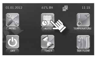
The **AUTO** mode enables scheduled operation of the ventilation unit. The unit runs at the pre-set speed and temperature during the specified time periods. The unit is in the Standby mode between the operating periods.
