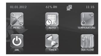
The Main menu contains the date, current humidity, time, temperature and set air flow.
