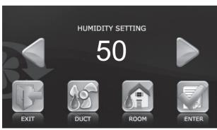
■ Select the humidity sensor type used to control the humidity:
