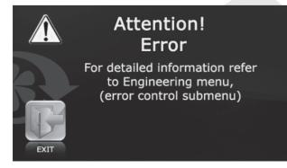
The control panel displays the following message in case of any malfunctions in the ventilation unit operation.
