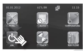
To turn the unit on/off press the **ON** / **OFF** buttons. Upon deactivation of the ventilation unit the icon changes from green to red.
