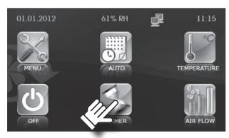
■ To activate the timer press **TIMER** in the control panel
