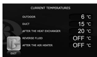
To review the current temperatures select the **CURRENT** TEMPERATURES submenu from the Engineering menu and press
