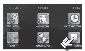
The MOTOR HOURS function enables the user to set up filter cleaning or replacement periodicity. Upon expiration of the pre-set time the panel displays a filter cleaning or replacement indicator. The indicator is displayed every 24 hours. Press the **RESET** button to reset the motor hours.
