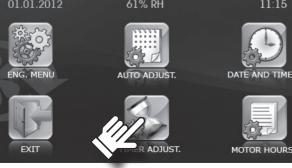
Activation of the **TIMER** function is confirmed with a tick If the AUTO and TIMER functions are activated synchronously, TIMER function will operate as it supersedes the **AUTO** function.
