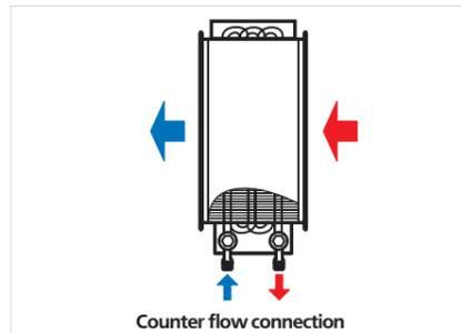
If water serves as a cooling agent, the coolers are suitable for indoor installation only in the premises with the indoor temperature not below 0 °C. For outdoor installation use an antifreeze mixture, i.e.ethylene glycol solution.
