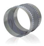
to the air duct as well as for the thermal distortion compensation within the air duct. Applied in ventilation systems with the transferred air temperature over the range of -40 °C to +80 °C. Compatible with round  $\emptyset$  100 up to 500 mm air ducts for VVG models and from  $\emptyset$  200 up to 630 mm air ducts for VVGF models.
