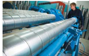
Spiral air ducts workshop
