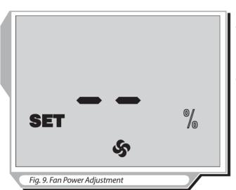
Upon entering the setup mode the panel display screen will show the SET and % indicators (Fig. 9).
