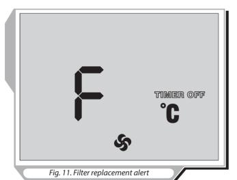
In case of filter replacement alert switch off the unit by pressing the button and disconnect it from the power mains. Replace the filters (see the sequence given in the "Technical Maintenance" section, page 14).
