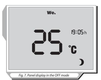
When the unit is off (Fig. 7) the control panel display indicates:
