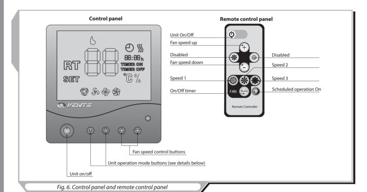
The unit is controlled by means of the remote-mounted control panel and the remote controller (Fig. 6).
