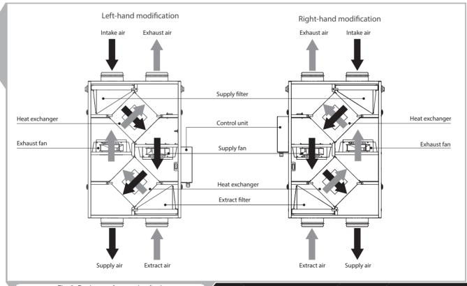
Fig. 2. Design and operating logic
