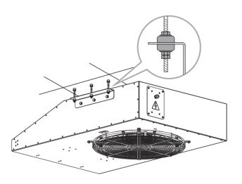
The fan is attached to the ceiling by means of specially designed mounting brackets. The fan is fixed to the ceiling in 6 points with expansion anchors or mounting studs.
