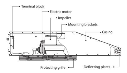
The fan casing is made of polymer coated steel. The protection grille on the air inlet side prevents ingress of foreign objects. The deflecting plates on the pressure side ensure equal air distribution and boost air draft.
