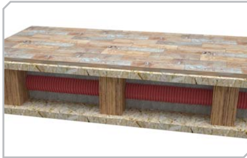
Inside wooden floor structures through the beams
