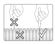
Cover the vents with caps to prevent ingress of foreign objects in the air ducts during mounting.
