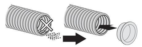
Use a sealing ring (available as a specially ordered accessory) on the air duct for airtight connection with the flange.
