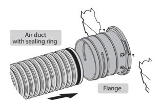
Use a lock ring (included in the delivery set of the flange) for reliable fixation of the air duct.
