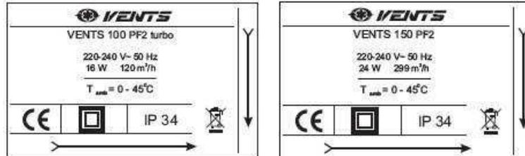
Design of rating label of other models is identical to the above except for type designation, rated power and flow rate
