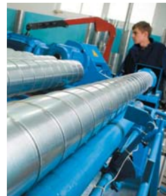
Spiral wound ducts workshop
