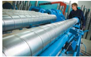
Spiral air ducts workshop
