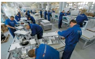
Air handling units workshop
