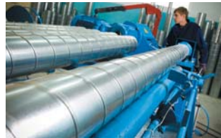
Spiral air ducts workshop
