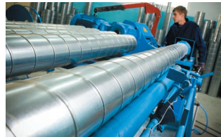
Spiral air ducts workshop
