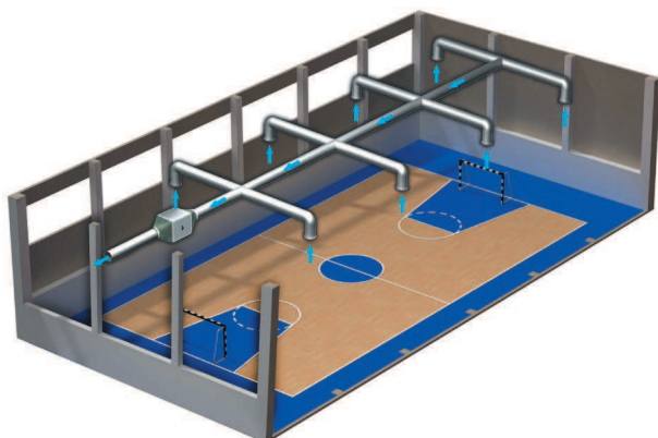
VS fan gym ventilation example
